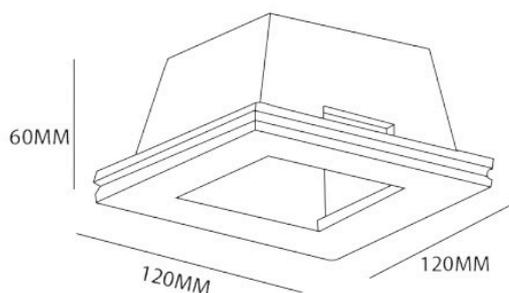
Led Downlight Plaster square 120x120 CO75mm closed IP44 white GU10 LH
