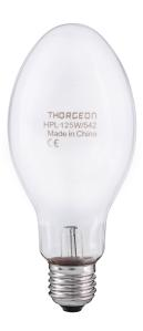
The Thorgeon HPL 125W mercury lamp is a reliable lighting solution for outdoor areas, warehouses, and industrial settings. Featuring an E27 screw base and a 4000K cool white light output, it delivers approximately 5900 lumens. With a lifespan of around 10,000 hours and a universal burning position, this lamp offers durability and versatility for various applications.
