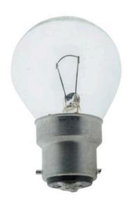
This clear B22d bulb with a G45 shape (70 mm length) operates at 24 volts and delivers 40 watts of power. It is ideal for use in 24V systems such as trucks, buses, and agricultural vehicles, as well as for signal lighting and low-voltage environments like boats or workshops. The bulb is dimmable with standard dimmers and has a lifespan of approximately 1000 hours.
