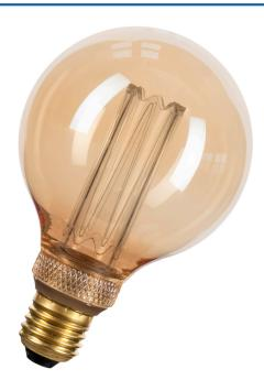
While a lot is already possible with the LED filament lamps, copying the super thin filaments of the original light bulb was still difficult. However, Bailey's Led Glow comes very close to it. The luminous and durable LED element is located in the lamp base. The "filaments" are engraved in an acrylic tube and reflect the warm 1800K light bulb color. The Led Glow really feels at home in a cozy environment.
