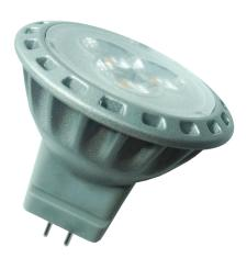
The so-called LED spots from the BaiSpot series are characterized by a much longer lifespan and significantly less energy consumption than their halogen predecessors. Due to the compact design, they are easily interchangeable. Spots are mainly used to provide directed light from the ceiling or wall. Wide voltage range: 24V-28V/DC or 12V AC/DC. Ambient temperature range: -20°C to +35°C.
