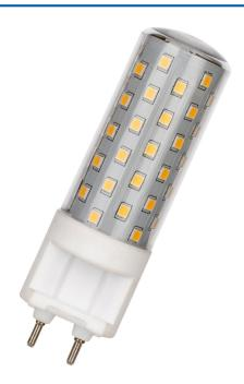
The compact LED G12 lamps are ideal as a replacement for ceramic metal halide lamps. These lamps are often used in shops, shop windows and museums. Installation: disconnect ballast, capacitor and igniter before use. Only suitable for temperatures up to 40°C inside the fixture. The LED light source can quickly malfunction due to overheating. Therefore not suitable for use in tight fixtures or fixtures where the reflector is close to the LED. Recommended to remove glass or cover from the fixture.
