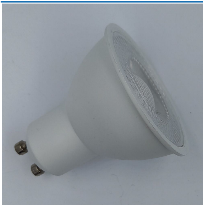
LED GU10 100-240V 50x56mm 5W 4000K 350Lm 36Degr. Toplux
